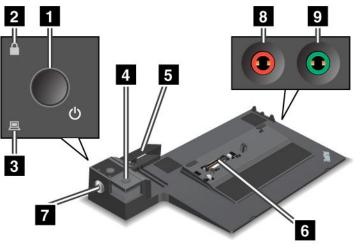
**1** Power button: Press the power button to turn the computer on or off.
